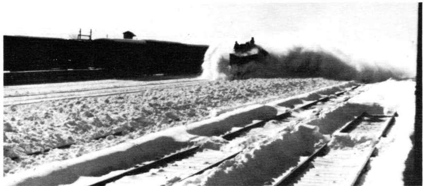
Here's a souvenir of winter, 1982 . . . spreader 799 working in Waterville Yard after one of our many storms.
