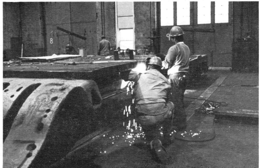
Lynn Fletcher and Steve Miles weld a section of a depressed flatcar at Waterville Shops. Ruth Brochu photo.
