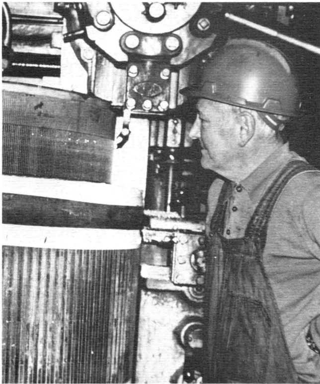
Machinist Rick Chamberlain turning commutator of main generator armature.
